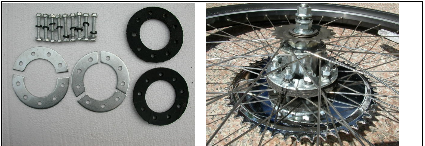
Figure #3 --- 9 hole - Chain Wheel Sprocket Installation mounted dish side inward:
